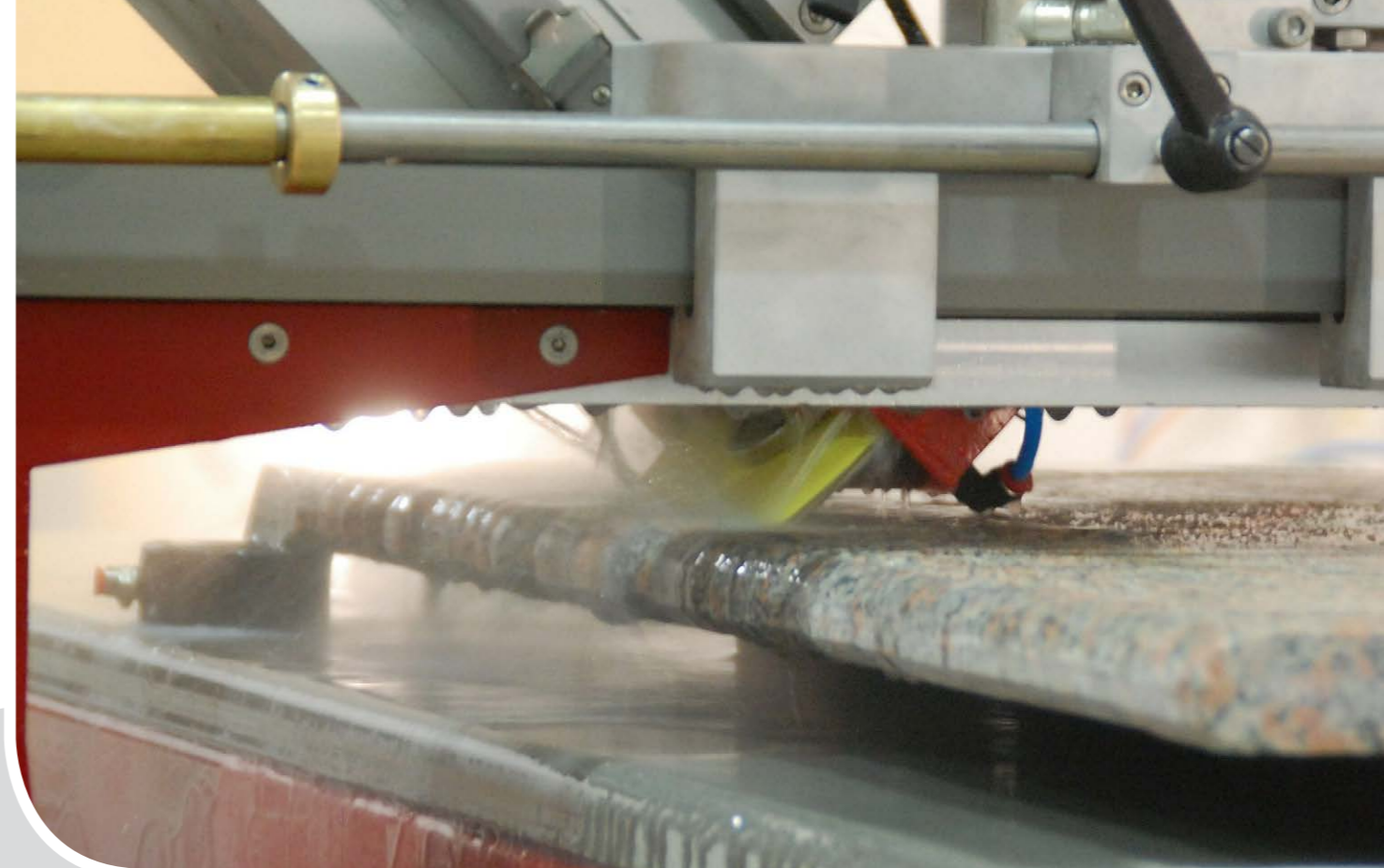
Inclined cuts at 45°
