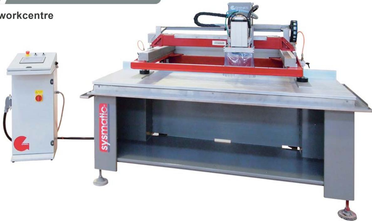
The Sysmatic **drills, cuts, shapes and polishes work pieces also longer than 3500 mm**. A software option allows to write and to engrave bas-relief. The reduced overall dimensions of the machine require only a small area and the installation is of very ease, without any structural works.
