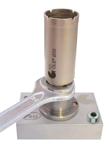
The base support helps to easily mount and dismount the tools onto the *Fast* tool holder
